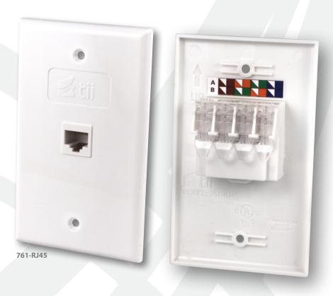
The Tii Indoor Flush Mount Ethernet Branded Jack is designed to provide a simple, fast, and reliable demarcation point for Ethernet services. It mounts to an industry standard single gang box and the rear CAT5e/CAT6 wire terminations are performed utilizing Tii's Industry Standard tool-less IDC connections.
