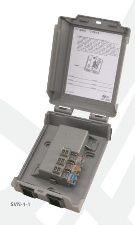
The Switchable Voice NID (SVN) contains a circuit that provides seamless switching from Telco service to digital phone service. The second ringing voltage appearance on the digital phone service initiates the switch over. The SVN utilizes gel-sealed insulation displacement terminations that provide reliable all weather connectivity. Flashing green LED indicates EMTA power is reaching SVN.
