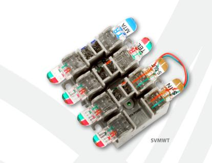
The Switchable Voice Module (SVMWT) provides seamless switching from Telco service to digital phone service. Available as a single switch module (with reset button) or a two-way switching module, the SVMWT provides a flexible design solution to meet individual customer needs. The SVMWT utilizes gel-sealed insulation displacement terminations that provide reliable all weather connectivity. A flashing green LED indicates EMTA power is connected to the SVM.
