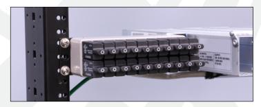
The P20 Series is a 20 pair protector unit designed to protect sensitive equipment on 20 copper pairs from overvoltage surge events. It utilizes industry standard 5 pin protector modules, and is typically installed in an OSP cabinet next to the 48VDC to High Voltage DC Upconverter for Line Powered applications such as Small Cell or 5G. Its space saving design is easily accommodated in most systems such as Alpha's CSM46 without occupying any additional rack space.
