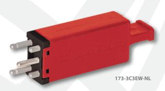
Tii gas tube modules are dependable plug-in devices that guard sensitive telecommunications systems from dangerous voltage surges. The gas tube utilizes a three-element design. This prevents destructive line-to-line over voltages, protecting PBXs and key systems in a way that conventional two-element gas tubes cannot.
