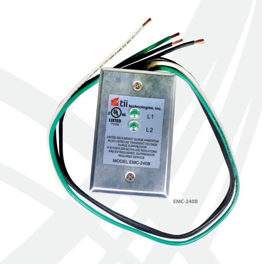
The **EMC-240B Surge Arrestor/Suppressor** is designed to protect powered OSP telecom cabinets, home electrical panels, or similar electronic equipment from destructive voltage surges. Wires exit from top of unit for easy panel mounting. Designed to be installed in standard two phase 120/240 Volt or single phase 110 Volt circuits. Front-facing LEDs indicate the protection circuitry is functioning properly.
