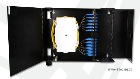
Wall mount fiber distribution unit designed to support patching and splicing in one unit. The enclosure has 4 adapter panel positions, allowing for a wide variety of fiber termination connector types. Two compartments separate the network terminations from the distribution terminations.
