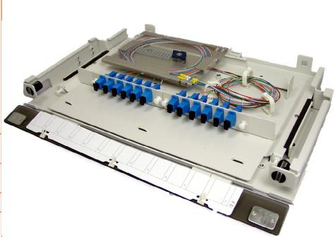
The RM1UWS is a fiber distribution chassis designed to support patching and splicing in one unit. The enclosure has 2 adapter panel positions allowing for a wide variety of fiber termination connector types and is equipped with a removable top cover. TSL shelves have been designed to meet Telcordia GR-63 and GR-449 Fiber Distribution Frame System requirements.
