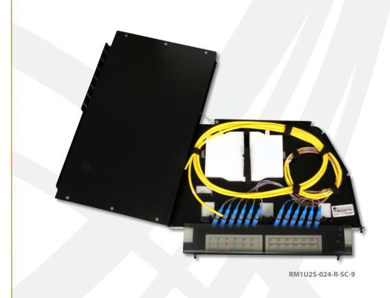
The RM1U2S is a 1 RU, 2 termination panel rackmount fiber distribution unit designed to support both patching and splicing in one unit. The enclosure has a swing out master panel that allows for easy access of terminations, fiber management and splicing.
