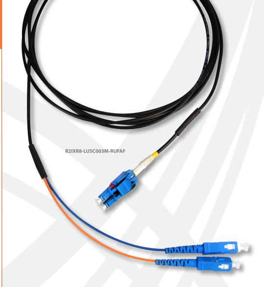
Duplex round outdoor rated 3mm patchcord terminated Compact LC-UPC uniboot connector for use in Remote Radio Unit applications. The round duplex cable and compact LC provide a single cable for easier cable management in tight spaces. Small diameter flexible weatherproof cable is composed of 2 tight buffer Singlemode optical fibers, water blocking aramid yarn, and UV resistant PVC jacket.
