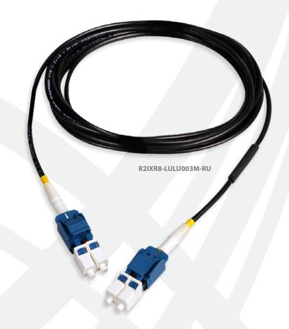
Duplex round outdoor rated 3mm patchcord terminated Compact LC-UPC uniboot connectors for use in Remote Radio Unit applications. The round duplex cable and compact LC provide a single cable for easier cable management in tight spaces. Small diameter flexible weatherproof cable is composed of 2 tight buffer Singlemode optical fibers, water blocking aramid yarn, and UV resistant PVC jacket.
