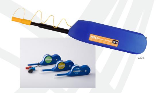
The US Conec IBC™ dry cloth ferrule cleaners are designed to effectively remove oil and dust contaminants that can negatively impact optical performance. The IBC cleaners can be used on unmated connectors such as cable assemblies or by removing the ferrule adapter; the unit will slide into an adapter and properly clean the ferrule behind a patch panel without having to remove the connector.
