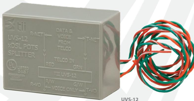
The UVS-12 POTS Splitter is a single line unit designed to be installed in series on the telephone line at the customer's premises providing a filtered POTS line connection for customer use. This POTS Splitter is designed to be used for all DSL services operating up to 30 MHz frequencies.
