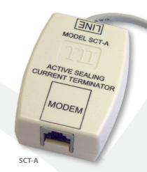
Tii's Active Sealing Current Terminator is a microprocessor controlled circuit that provides DC sealing current terminations to non telephone service DSL subscriber lines. It maintains network connection integrity by allowing current to flow through "DSL Only" service.
