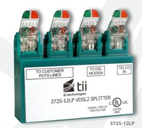
The 372S-12LP DSL POTS Splitter Module splits the combined voice and data signals carried on telephone lines providing separate outputs for both phone and data services. This splitter module utilizes enhanced circuit components to meet VDSL2/ADSL2+ splitter specifications for advanced data and IPTV deployments.
