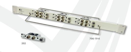
The 706 Series DS-3 Protector Panel accommodates the 202 Series coax rack mount modules. The panel can accommodate up to six 202 Series modules which consists of 12 coax protectors. Designed specifically for today's high speed digital coax distribution networks, Tii's state-of-the-art DS-3 Protector Panel protects personnel and equipment from lightning and power-induced overvoltage surges on coaxial cable circuits.
