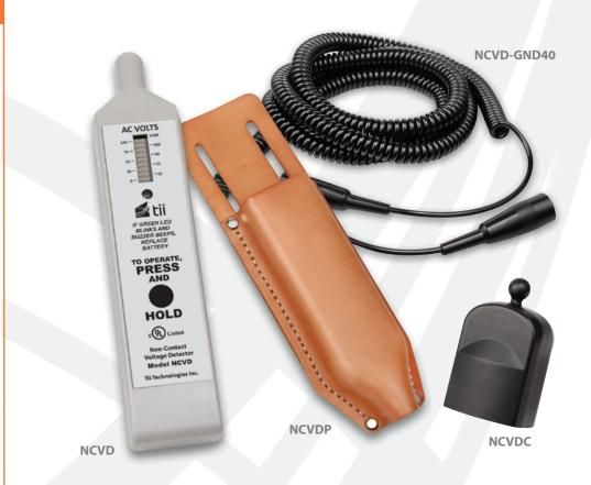
The Non-Contact Voltage Detector (NCVD) allows a communication technician to test a work location for the presence of potentially hazardous Alternating Current voltages. The NCVD detects the presence of the electric field associated with a live circuit without making contact to the wire or device under test. The NCVD is molded out of insulating thermoplastic material to further reduce the risk of exposure.
